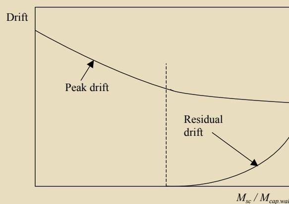
**Figure 1.** This graph plots the drift versus relative strength of the resisting elements. Source: Stanton and Nakaki 2002. Note:  $M_{cap.wall}$  = total moment capacity of wall;  $M_{sc}$  = total moment capacity of all U-shaped flexural plate connectors.
