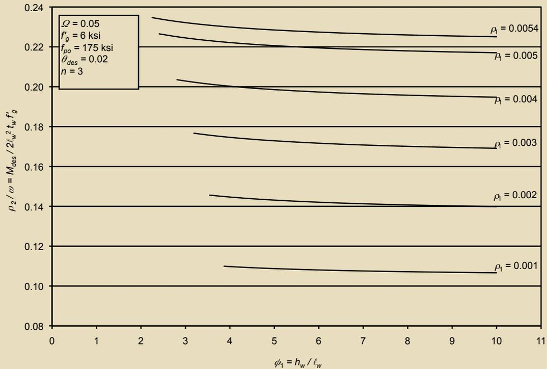
**Figure 9.** This graph plots  $\rho_2/\omega$  versus  $\phi_1$  for three wall panels ( $n = 3$ ) and  $\Omega = 0.05$ . Note:  $n$  = number of wall panels per wall;  $\phi_1$  = ratio of  $h_w$  to  $\ell_w$ ;  $\rho_2$  = ratio of  $F_{sc}$  to  $\ell_w t_w f'_g$ ;  $\Omega$  = ratio of  $h_w(\gamma_c + \gamma_d)$  to  $f'_g$ ;  $\omega$  = ratio of the moment resisted by the shear connectors to the total design moment.
