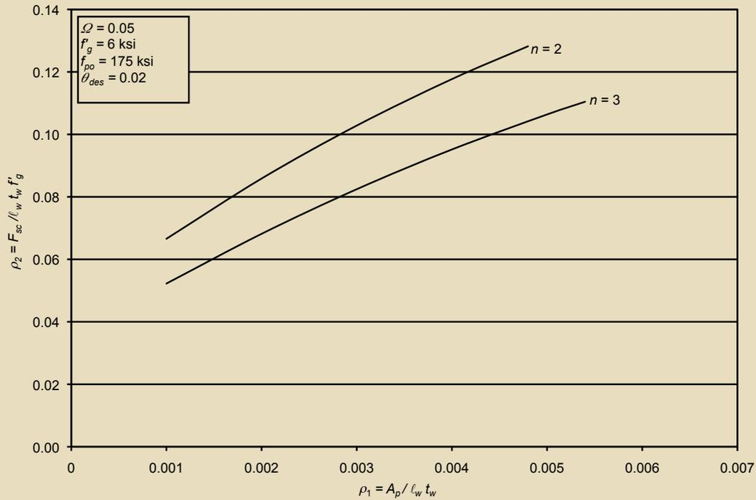
**Figure 10.** This graph plots  $\rho_2$  versus  $\rho_1$  for  $\Omega = 0.05$ . Note:  $\rho_1 =$  ratio of  $A_p$  to  $l_w t_w$ ;  $\rho_2 =$  ratio of  $F_{sc}$  to  $l_w t_w f'_g$ ;  $\Omega =$  ratio of  $h_w(\gamma_c + \gamma_d)$  to  $f'_g$ .
